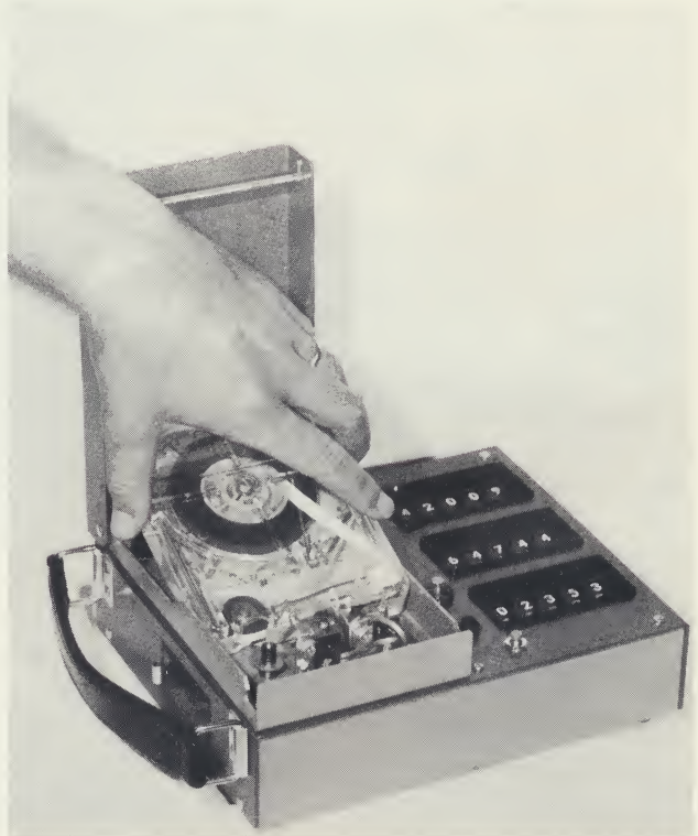
Magnetic tape cartridge being inserted into Hand Recorder.
